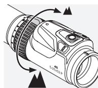
You can set the desired magnification by turning the (stepless) magnification adjustment ring through 180°. The scale on the adjustment ring allows simple and easy reading of the setting. The soft, ribbed covering of the adjustment ring has a nose for better orientation. When the magnification is changed, the aiming point and windage marks position will adapt accordingly.
