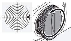
b) ... counterclockwise for a shot to the right for the required impact point correction (1/4 MOA; 7 mm/100 m or 0,25 in/100 yds)
