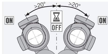
The reticle illumination and display turn off after 40, 60 or 80 seconds (the time can be pre-set in the App). A warning signal appears 10 seconds in advance. Press the +/- button or tip the dS by 20 degrees left or right to increase the display duration by the pre-set period of time. If the display turns off, the measurement button must be pressed again to activate it.
