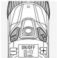
To turn on the reticle illumination, press the plus/minus buttons simultaneously for half a second.
