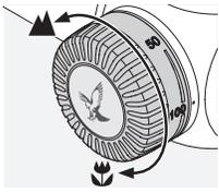
Using the parallax turret, you can adjust the optimum focus for every target distance thus preventing aiming errors due to parallax. The parallax turret can be set from 50 m to infinity.
