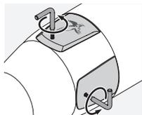
2. The covers of the elevation and windage adjustment can be opened with the provided torx screwdriver (TX 6). You can then adjust the elevation and windage adjustment when open with the adjusting tool.
