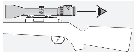
Please note the eye relief distance specified for a mounted rifle scope (see technical data sheet for dimensions).
