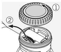
1. Open the battery cover and remove the torx screwdriver and the adjusting tool.
