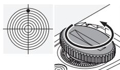
b) ... counterclockwise if the shot is high for the required impact point correction (1/4 MOA; 7 mm/100 m or 0,25 in/100 yds).
