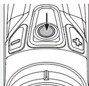
An illuminated circle, the aiming mark, appears after you press the measurement button and the measuring function is activated. If you release the measurement button, the measurement is triggered and the aiming point calculated from your entered data will appear. The reference mark is the central aiming point of the physical reticle.
