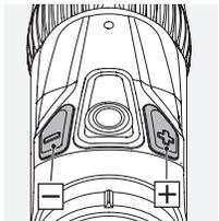
Once the reticle illumination is turned on, you can now adjust the brightness by means of the +/- buttons and select the setting of your choice from among 64 brightness levels. Keep the button pressed (constant impulse) to rapidly find the optimum brightness, to adjust finely press the button once (single impulse).
