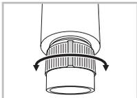
By turning the ocular you can focus any object sharply at a distance of 10 m / 33 ft to infinity. In the infinity position the little nose on the ocular is at the top.
