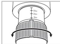
On the ocular you find a scale for the estimation of distance. This scale is designed for easy focusing.
