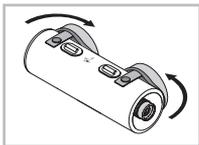
The lens and eyepiece are protected against dirt and damage by caps.
