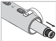
Hold the body and the ocular of the extendable telescope firmly and then pull outwards until the extension reaches its stopping point.
