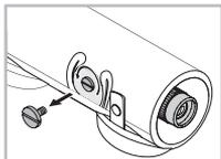
The tripod base has a connecting thread of 3/8" UNC. The inserted bush reduces the connecting thread to 1/4". The observation telescope thus fits on any standard tripod.
