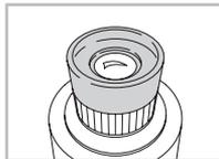
By turning back the eyecups, the eyeglass-wearer can optimally utilize the full field of view. The eyecups can be unscrewed for cleaning or replacement.
