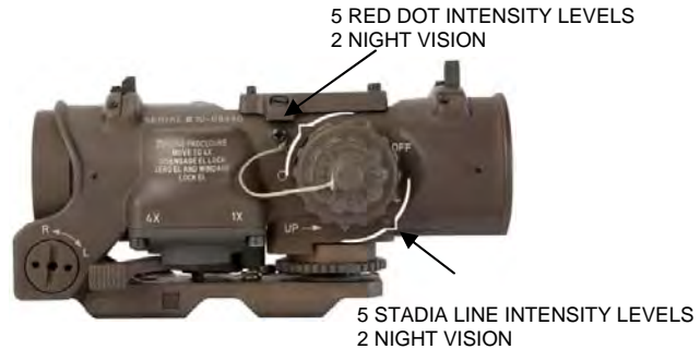
Figure 3-4: Reticle Illumination Switch Operation - rotate the switch to desired reticle brightness setting.
